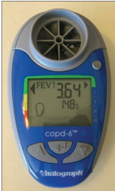
Figure 1. The Vitalograph copd-6™ pocket spirometer detects airway obstruction from six-second FVC manoeuvres using FEV1/FEV6 and FEV1 % predicted. Three manoeuvre quality checks are performed in order to reduce the risk of misclassification, due to submaximal efforts.
