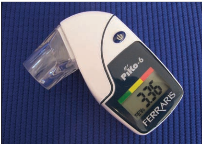
Figure 3. The nSpire PiKo-6™ is the smallest pocket spirometer, measuring FEV1, FEV6, and FEV1/FEV6 (but not predicted values) from six-second forced vital capacity manoeuvres. An optional base sends the numeric results (but not graphs) to a personal computer.
