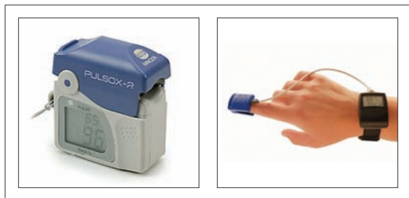
Figure 2. Two types of oximeters from reputable manufacturers. a) The Minolta PulseOx-2 is used for spot-checks, whereas b) the Nonin 3100 WristOx can be used for serial monitoring.
